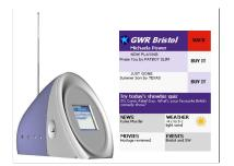
This rather odd thing did similar. This was a project run by GWR FM in Bristol, and the radio picked up additional content broadcast via DAB, and also connected to wireless internet. You can see the touch screen on the right.
